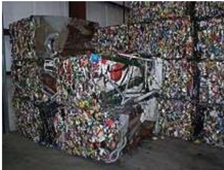
Fig. 5.7: Steel Crushed and Baled for Recycling
