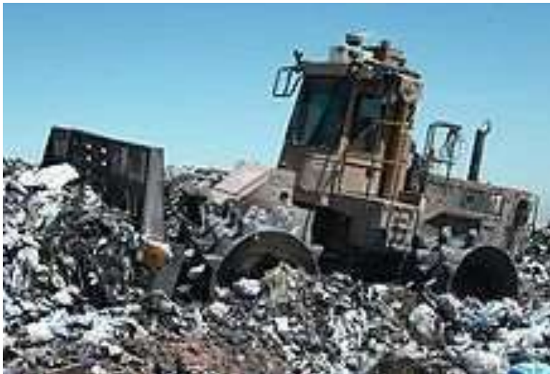
Fig. 5.3: A Landfill Compaction Vehicle in Action
